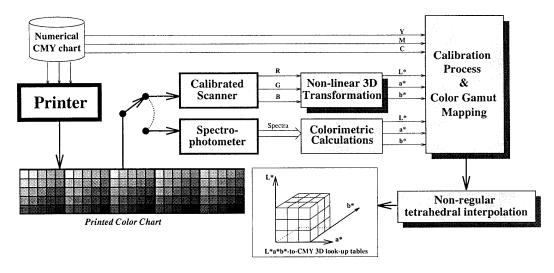
Figure 4. The printer calibration process, providing a 3D lookup-table for the conversion from CIELAB to CMY.
