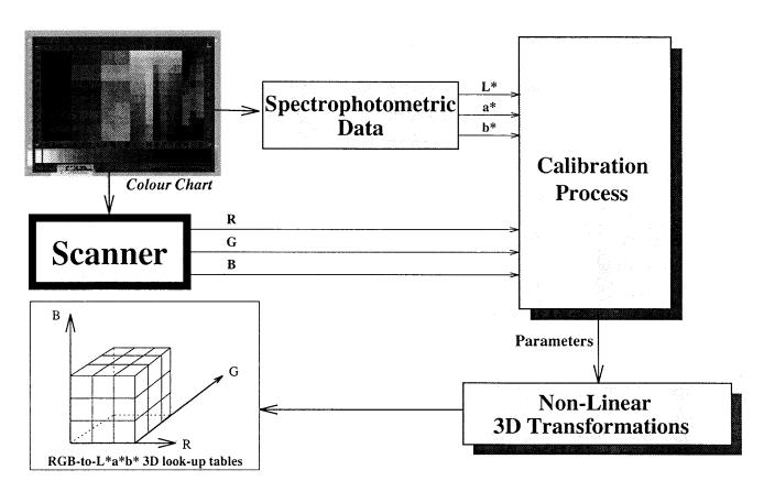
Figure 2. The scanner calibration porcess, providing a 3D look-up table for the conversion from scanner RGB to CIELAB.
