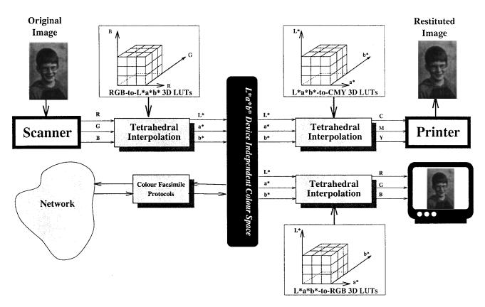
Figure 1. A color facsimile system. The transformations between device dependent color coordinates (RGB and CMY) and the CIELAB color space is performed using 3D look-up tables and a tetrahedral interpolation technique.
